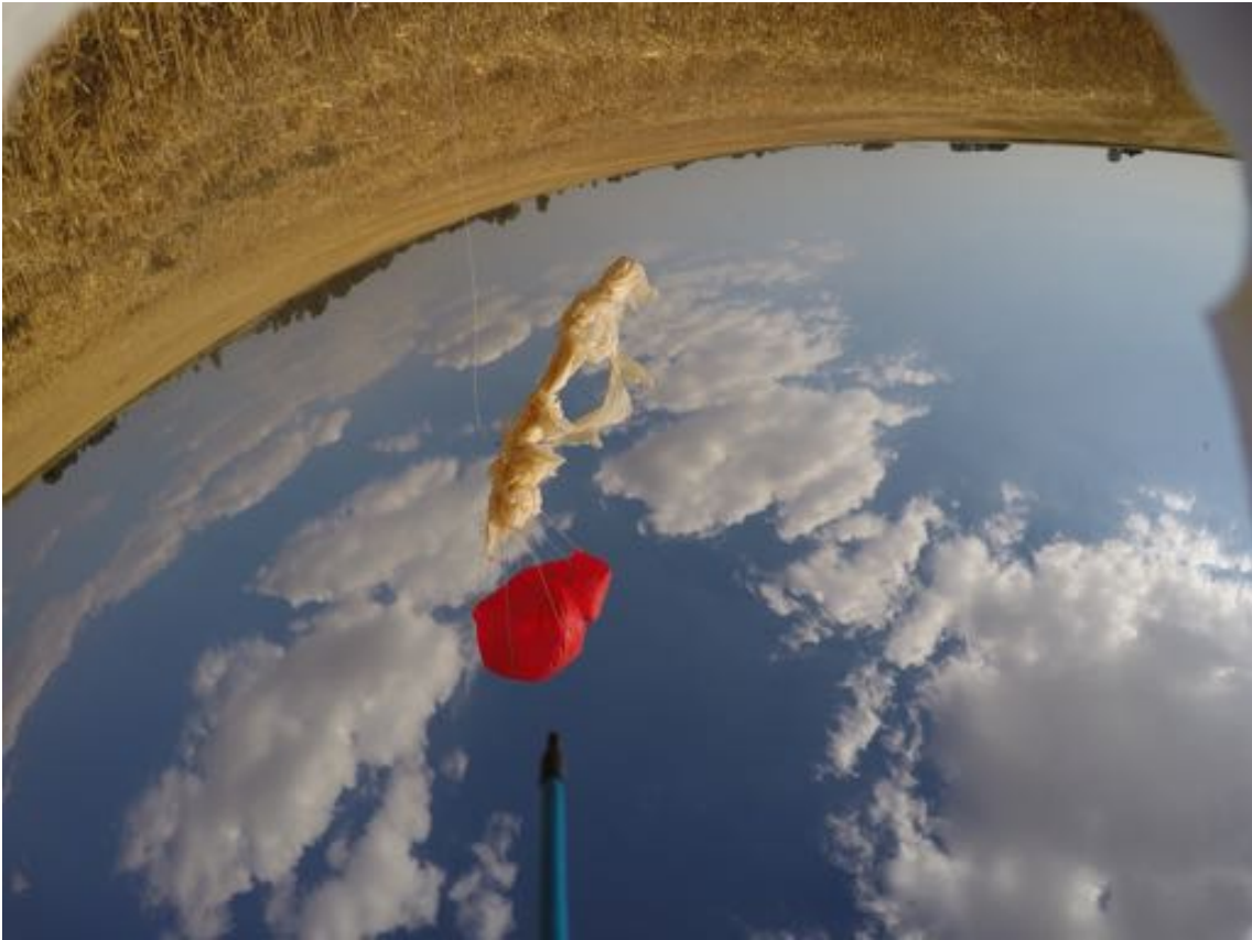
Figure 8: Titan's parachute with balloon remains wrapped around the parachute's lines. This image proves that the parachute opened during descent, even if not fully.
